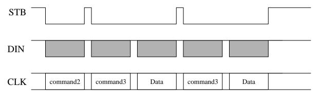
Where : Command 2 -- Data Setting Command Command 3 -- Address Setting Command Data -- Display Data
