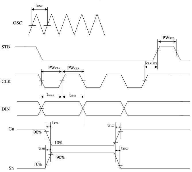
PW <sub>CLK</sub> (Clock Pulse Width) ≥400ns t setup (Data Setup Time) ≥ 100ns t <sub>CLK-STB</sub> (Clock - Strobe Time) ≥ 1 $\mu$ s t <sub>TZH</sub> (Rise Time) ≤ 1 $\mu$ s t <sub>TZL</sub> <1 $\mu$ s
