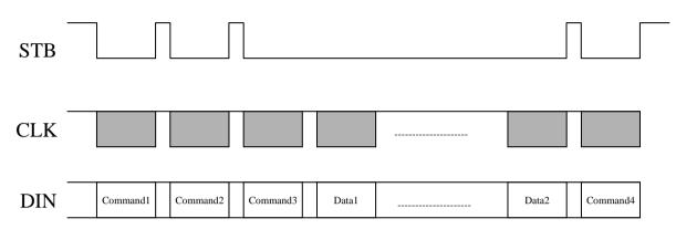
Where : Command 1 : Display Mode Setting Command 2 : Data Setting Command Command 3 : Address Setting Command Data 1 to n : Transfer Display Data (14 Bytes max.) Command 4 : Display Control Command
