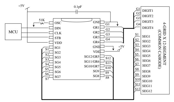
Note : The capacitor (0.1uF) connected between the GND and VDD Pins must be located as near as possible to the KK1207 chip.
